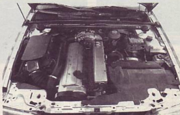
Motor: 5 valjev, 20 ventilov, overboost, 230 KM
